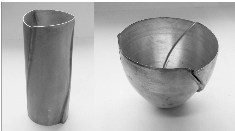
Figure 22 Rotating the form while traversing creates twisted forms.
