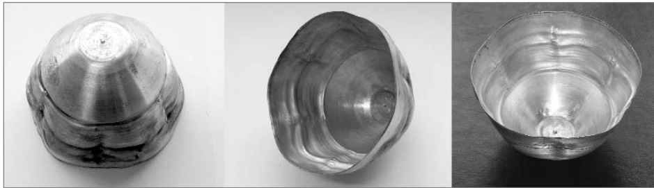
Figure 23 Using laser forming to create forms with undercuts.
